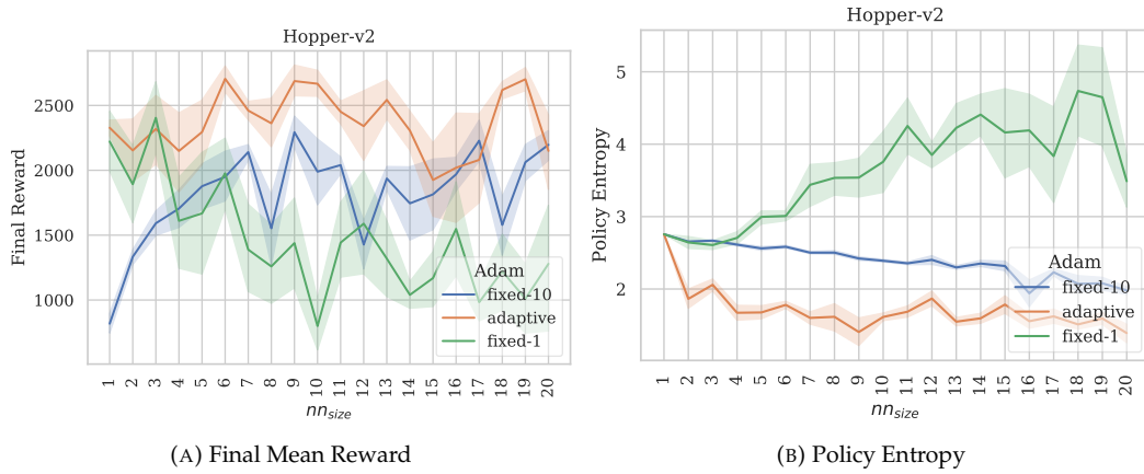
FIGURE 4.15: The final mean reward (left) against the final policy entropy (right). Both graphs represent the average taken over the last ten policy updates. An insufficiently large step size does not affect the entropy of the policy, which we can read for fixed-10 in the interval n_{sizes} \in \{1, \dots, 7\} .
